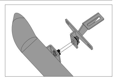
3. Depending on your year model, there will be either existing 8mm threaded holes for the M8 Hex Head Bolts or open slots for the M10 Speed Clips.
