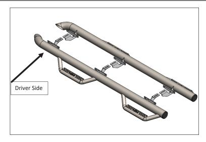
2. Using M10 Carriage Bolt and M10 Flanged Nut, loosely attached mounting brackets to Nerf-step.
