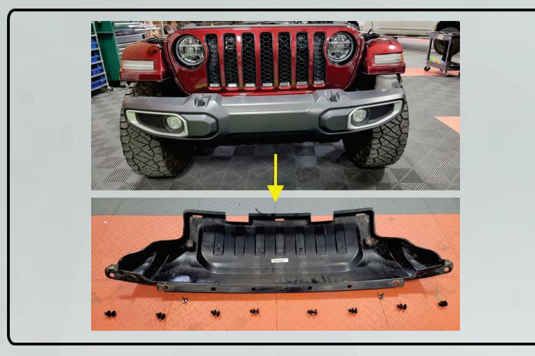
2. Remove the six (6) plastic clips holding the fog light cover behind each fog light. Remove and set fog light covers aside.
