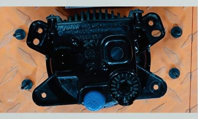
4. Connect the Deutsch DT to 5202 adapters to the factory connectors. Ensure the connector lock is engaged.
